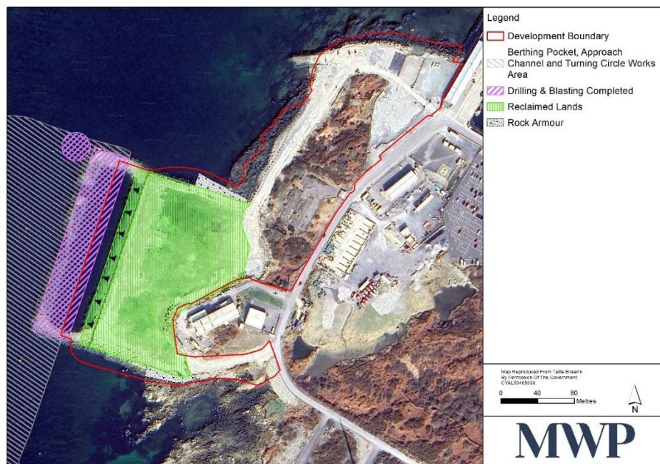
Figure 4: Map of the development works area, including the reclamation area, the blasting and dredging areas, the berm construction areas and rock armour placed undertaken between Jan 2023 and May 2024.
